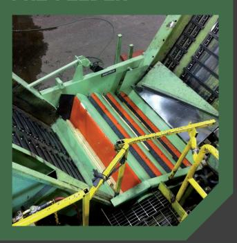
Novilco's automatic stick infeed system will keep up with your stacking operation at any speed. It's a reliable, efficient, fully automated system which requires minimum operator intervention.
