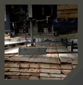
The Novilco Falcon Stick Placers are an integral part of the high speed stick placing system designed to significantly increase efficiency and eliminate bottlenecks in the stacking section of sawmills.
